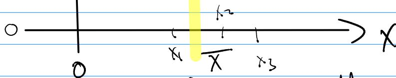
$$\bar{x} = \frac{\sum_{i=1}^n M_i x_i}{\sum_{i=1}^n M_i} = \frac{\text{Moment from } (y \text{-axis})}{\text{total mass}} = \frac{M_y}{M}$$
