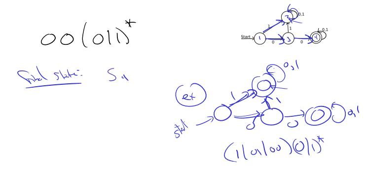
8) Determine the language recognized by a given non-deterministic finite-state automaton.
